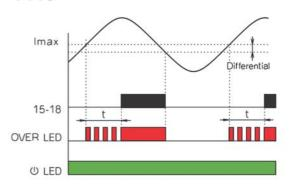
The time delay and differential trip levels help to prevent relay chatter as the monitored current level varies. As the relays have changeover contacts, the relay outputs can be inverted by wiring to the alternative terminals 15-16 or 25-26.
